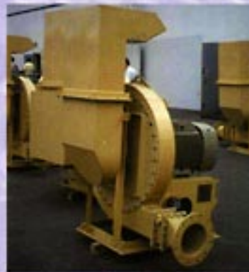
Elbow Inlet Box silencer on Fan Equipment Blower
